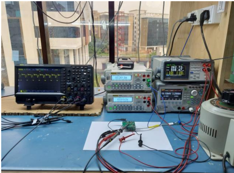
Figure 4: 45 W QRF EVB test setup.
