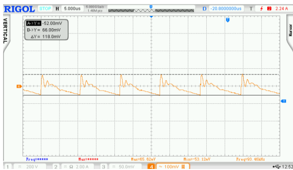
Peak-to-Peak Ripple 118mV at 20V output.
